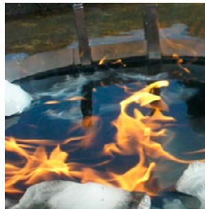
Laser ignition and self-sustaining combustion on various surfaces: on ice, on water under snow, on open water and on sand
