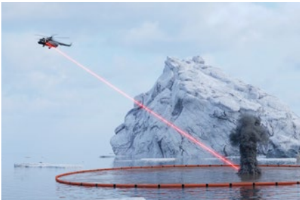
Laser ignintion of oil from the air
