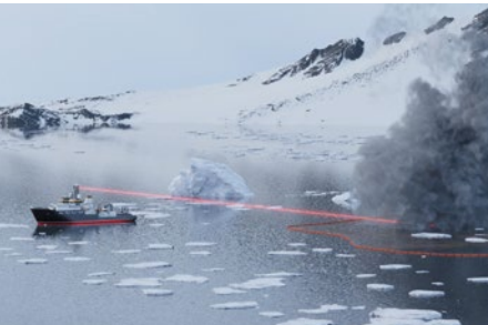
Laser ignition of oil from a ship
