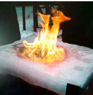
Laser ignition and self-sustaining combustion on various surfaces: on ice, on water under snow, on open water and on sand
