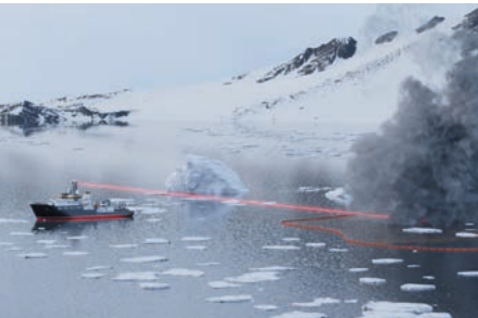
Laser ignition of oil from a ship
